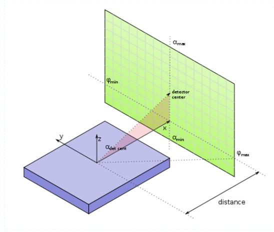
Figure 4.1: Experimental geometry with a two-dimensional pixel detector.
