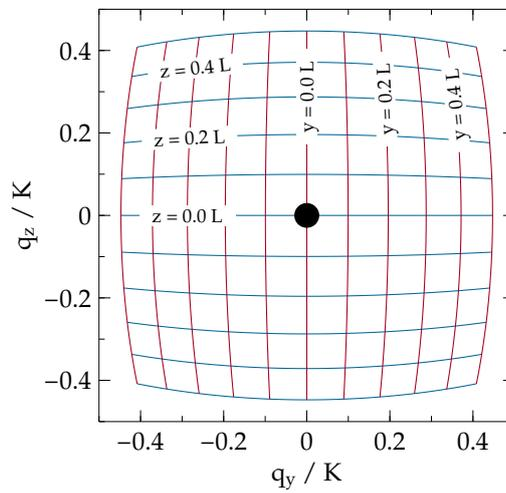
Figure 4.5: The outer contour of the blue and red grid shows the border of a square detector image after transformation into the physical coordinates  $q_y, q_z$ . The blue and red curves correspond to horizontal and vertical lines in the detector.
