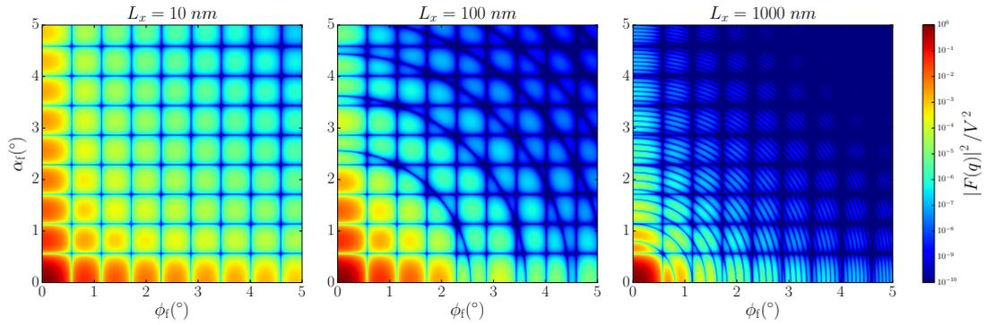
Figure 4.4: Simulated detector image for small-angle scattering from uncorrelated cuboids (right rectangular prisms). The incoming wavelength is 0.1 nm. The prisms have edge lengths  $L_y = L_z = 10$  nm; the length  $L_x$ , in beam direction, is varied as shown above the plots. The circular modulation comes from a factor  $\text{sinc}(q_x L_x/2)$  in the cuboid form factor, with  $q_x$  given by (4.4).
