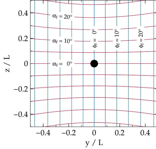
Figure 4.2: Lines of constant  $\alpha_f$  (red) or  $\phi_f$  (blue) in the detector plane, for a planar detector at distance  $L$  from the sample. The black dot indicates the beamstop location for the central incident beam (SAS geometry,  $\hat{\mathbf{k}}_i = \hat{x}$ ).
